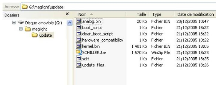
Insert the USB key in the connector **(15)** provided, select the update button and loading will start automatically. Follow the instructions. At the end of the loading process, the device will go off automatically.
