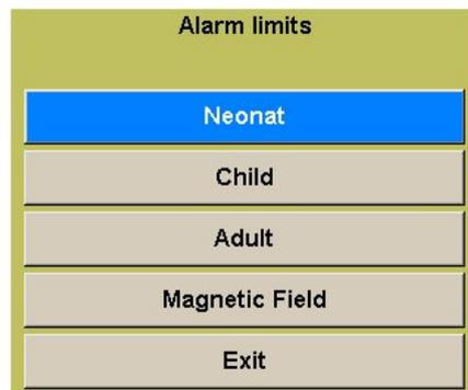
Select the parameter by navigation button **(6)** counter clockwise and confirm by pressing button **(6)**. The first value will flash. Turn as required to modify the value. Save the value by pressing button **(6)**. The next value is automatically selected. When the last parameter value has been entered, the selection cursor goes back to the parameter selection column.
